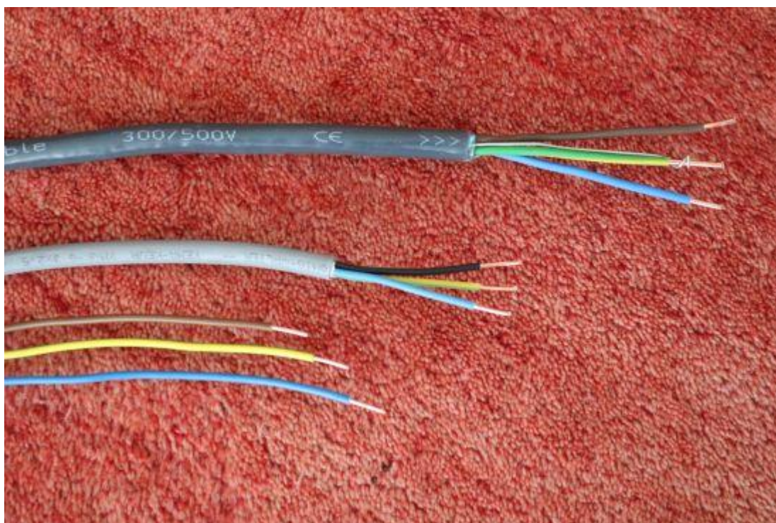
From top to bottom: GigaWatt LC-Y-EVO in-Wall cable, XMVK double-isolated 2,5 mm 2 solid-core installation wire and 2,5 mm 2 regular solid-core installation wire
