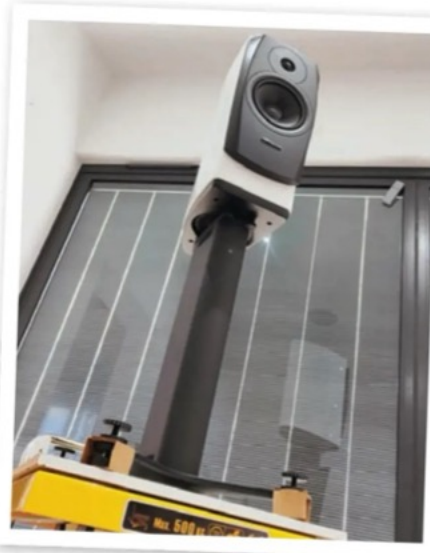
ABOVE: Lifting speakers clear of reflective boundaries is crucial in obtaining a long 'anechoic' time window for our lab tests. Here's Dynaudio's Confidence 20A [p76] on its way up...
