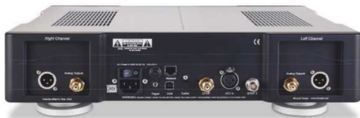
ABOVE: Supported digital inputs include wired Ethernet (as a DLNA compatible network player the M21 handles up to 384kHz PCM, native DSD64 and DSD128 over DoP), USB-B (also 384kHz PCM and DSD128), optical/coax S/PDIF and AES/EBU (XLR)
